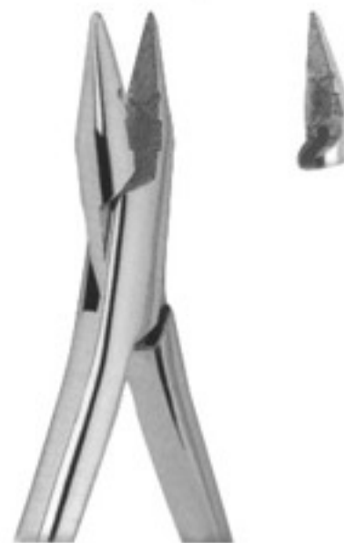
3214 Nance Universal pliers for bending wires up to 0,9 mm. (.035") or cutting up to 0,7 mm. (.028").
